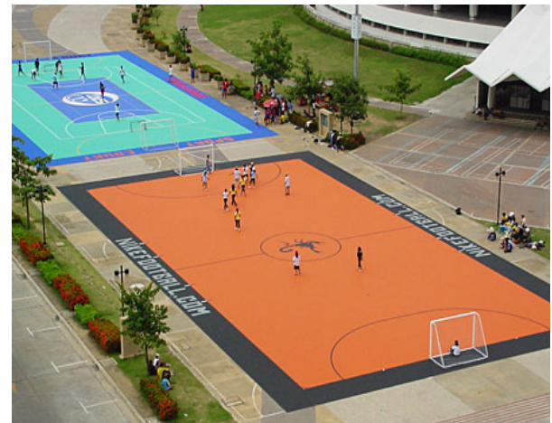
Figure 4. Multi-sport surface made from tile floor
