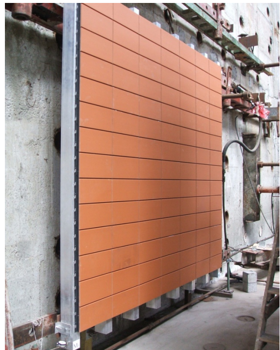
Photo 8 Type A specimen made up of Tonality classic 25/200/400 tiles type during loading
