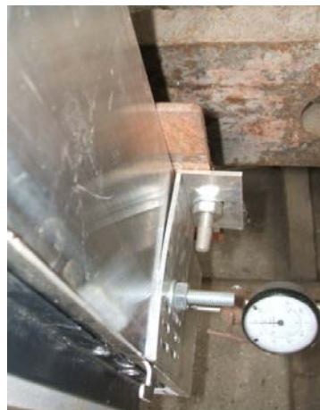
Photo 1 Monitoring displacements at the lower side of the specimen
