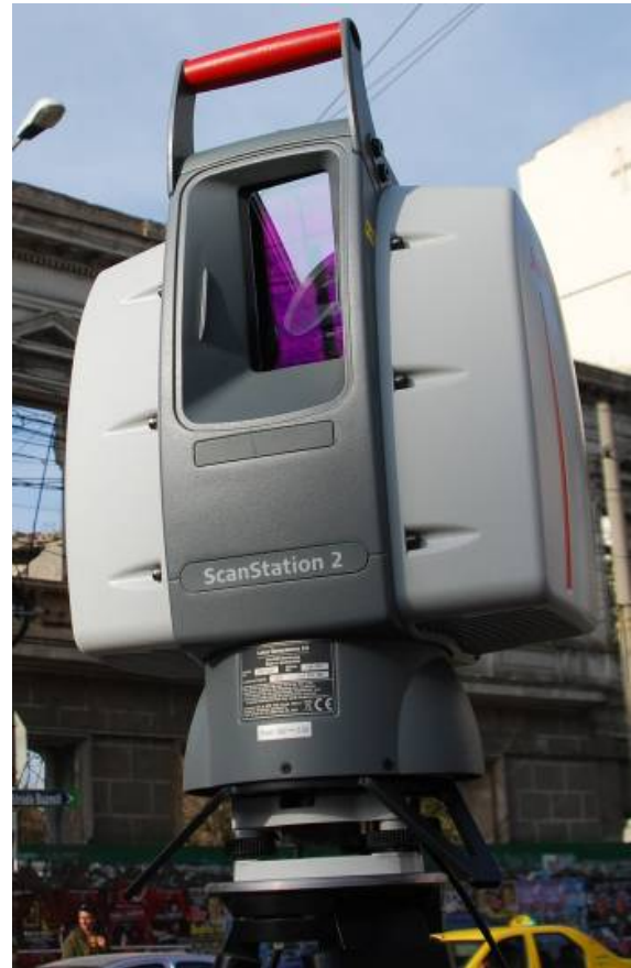
Figure 3. Leica SCANSTATION 2 laser scanning system
