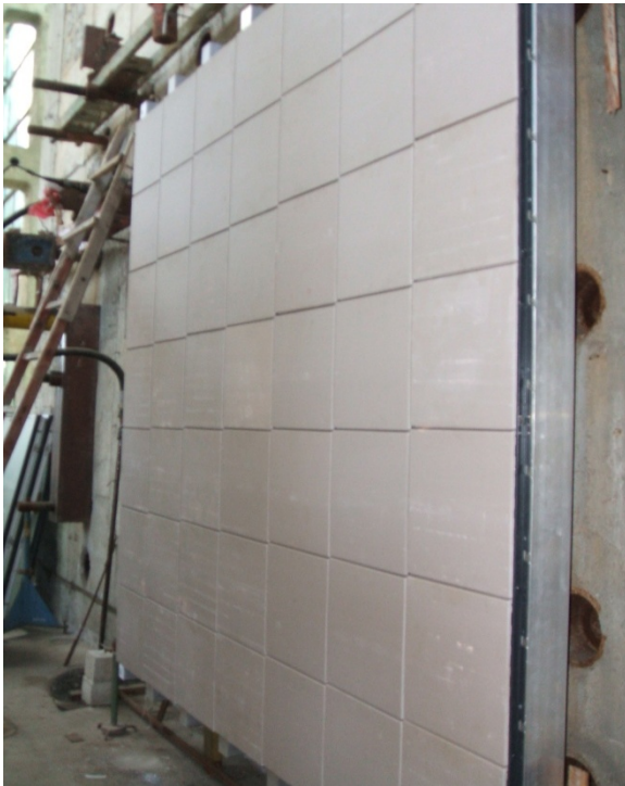
Photo 6 Type A specimen made up of Tonality classic 25/200/400 tiles type during loading.
