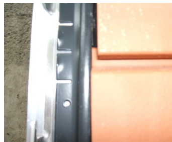
Photo 3. Relative rotations and displacements between facades tiles at maximum drift of 3%
