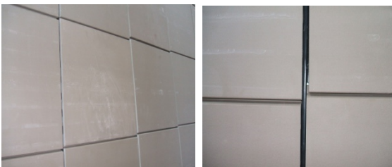
Photo 7 Relative rotations and displacements between facade tiles at maximum drift of 3%
