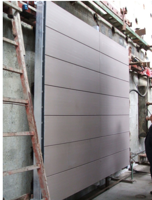
Photo 4 Type A specimen made up of Tonality classic 25/200/1500 tiles type during loading.
